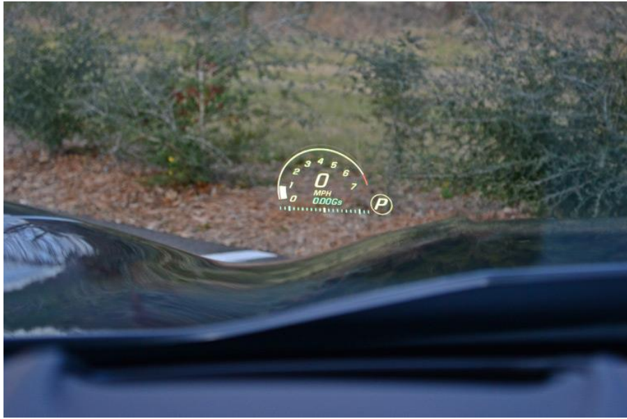
Figure 1: The Heads Up Display of a Chevrolet Corvette, displaying a tachometer, speedometer, and g-meter.
