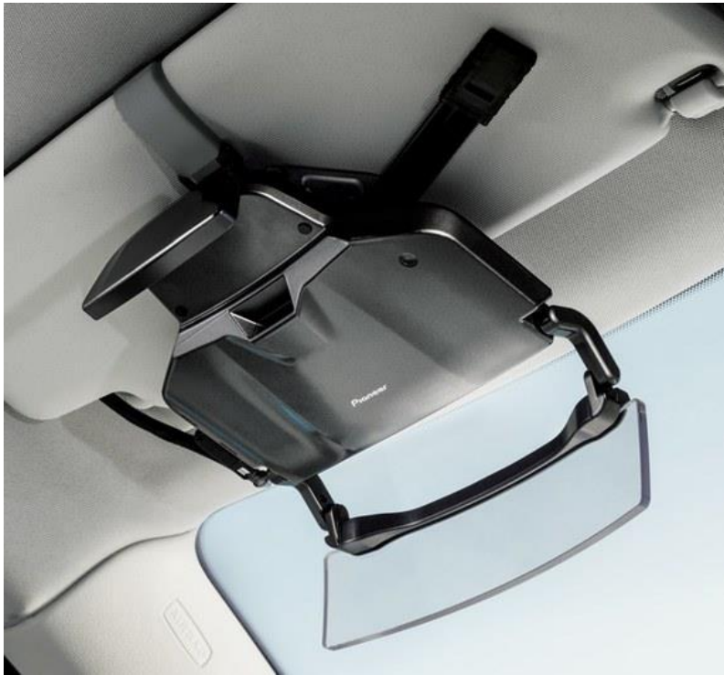
Figure 5: An off-the-shelf GPS heads up display that features its own display screen.
